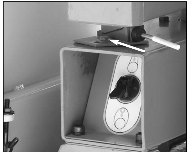
Figure 23. Loosen these bolts to adjust the limit switch position.
